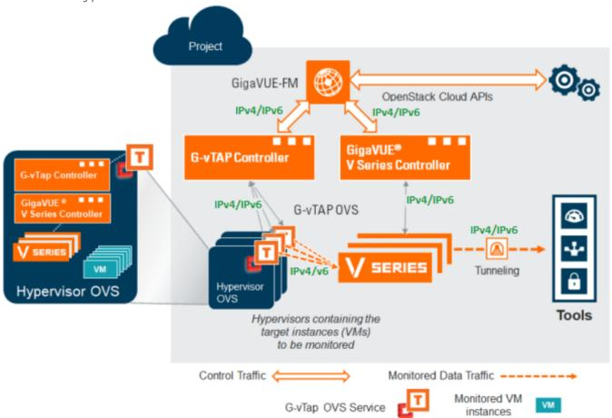
The G-vTAP Agents are deployed on the target hypervisors and the configuration file is to be modified based on the requirements and service. GigaVUE-FM connects to G-vTAP Controller and each G-vTAP Controller can talk to G-vTAP Agents. GigaVUE-FM receives the list of interfaces that can be used as the source or destination for the mirroring interface selected in GigaVUE-FM. GigaVUE-FM mirrors and forwards the traffic to the V Series nodes based on the deployed Monitoring Session.
