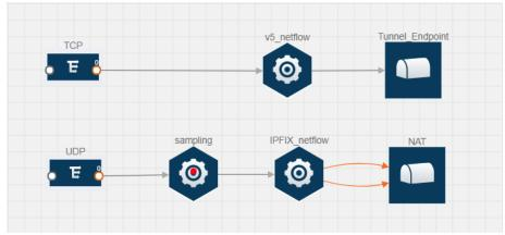
The NetFlow record generation is performed on GigaVUE V Series node running the NetFlow application. In Add Applications to Monitoring Session, incoming packets from G-VTAP Agents are sent to the GigaVUE V Series node. In the GigaVUE V Series node, one map sends the TCP packet to the version 5 NetFlow application. Another map sends the UDP packet to a sampling application. The map rules and applications such as slice, mask, and sample can only be applied prior to sending the data to NetFlow.
